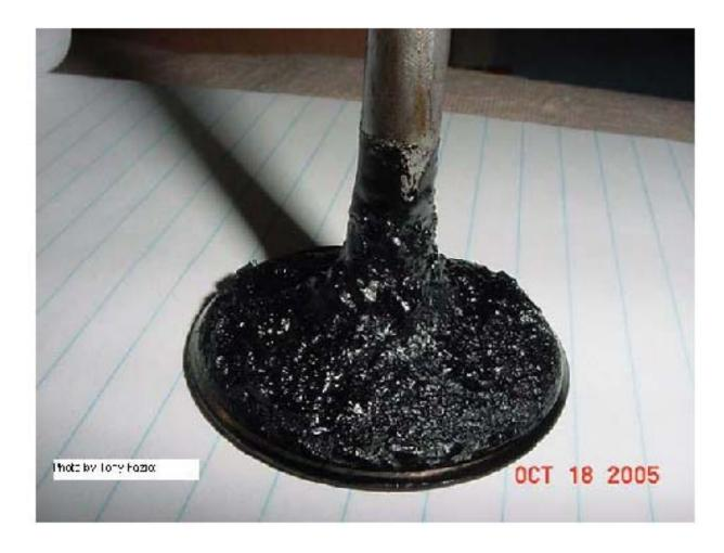
Valve with carbon build-up from breakdown of the resin in fiberglass fuel tanks.
