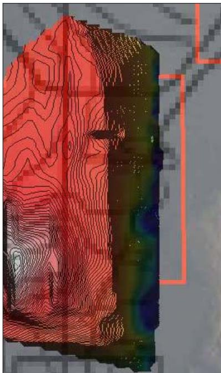
Figure 3-2. Color-coded contour plot of magnetic data recorded during the 2009 geophysical survey of the NBHSS shipwreck study area (image courtesy of CRE).
