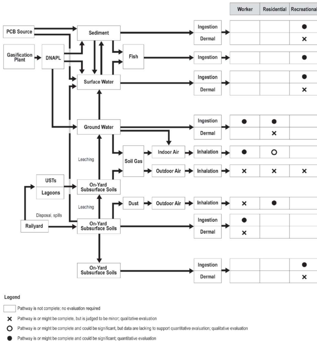
Figure 2-4. Example Conceptual Model of Exposure Pathways for Multiple Receptors to Multiple Stressors for Superfund Site Assessment
