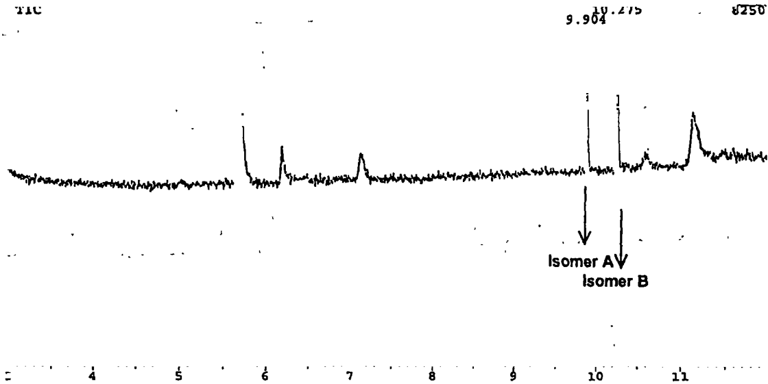
Figure 1 : Chromatogram matrix standard solution KWG 4168 10 µg/L (Chromatographic conditions A)
