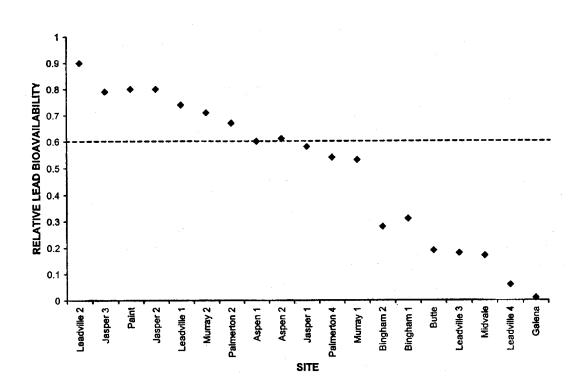
**Figure 4.** Swine feeding studies using 17 field soils contaminated with lead and two laboratoryprepared soils (paint in soil and galena in soil). The dashed line represents the 60 percent relative bioavailability used to set the national default value for absolute bioavailability of lead in soil used by EPA (Henningsen et al., 1998a).
