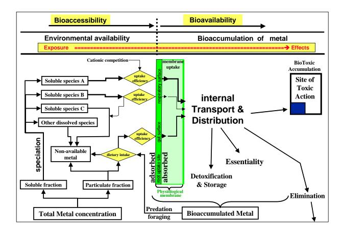
**Figure 1.** Conceptual diagram of processes controlling the bioavailability and the bioaccumulation, both toxic and benign, of metals from the environment. Note that complexation and the speciation of metals is illustrated by dissolved species A, B, C, and other, and that the relative bioavailability of these is represented via the thickness and endpoint of the arrows leading from the respective boxes.
