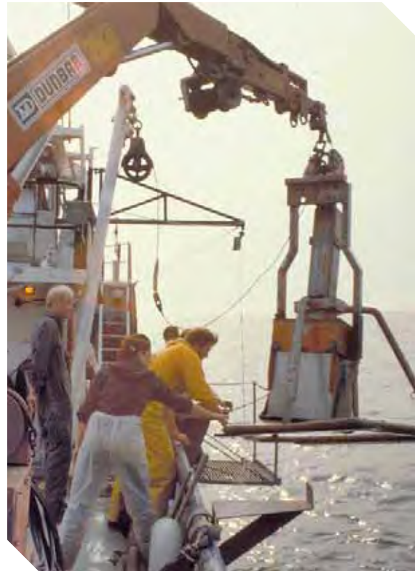
Box core samplers are used to collect sediment samples from the lake bottom without disturbing the surface (courtesy of U.S. EPA).
