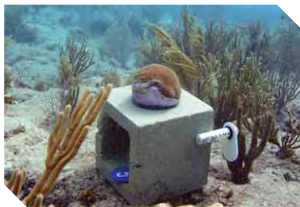
This monitoring station measures calcification rates to determine the impact of ocean acidification on coral growth at Fowey Rocks Light Reef in Biscayne National Park, FL (courtesy of USGS).
