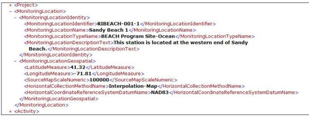
Figure 4. <MonitoringLocation> data elements.
