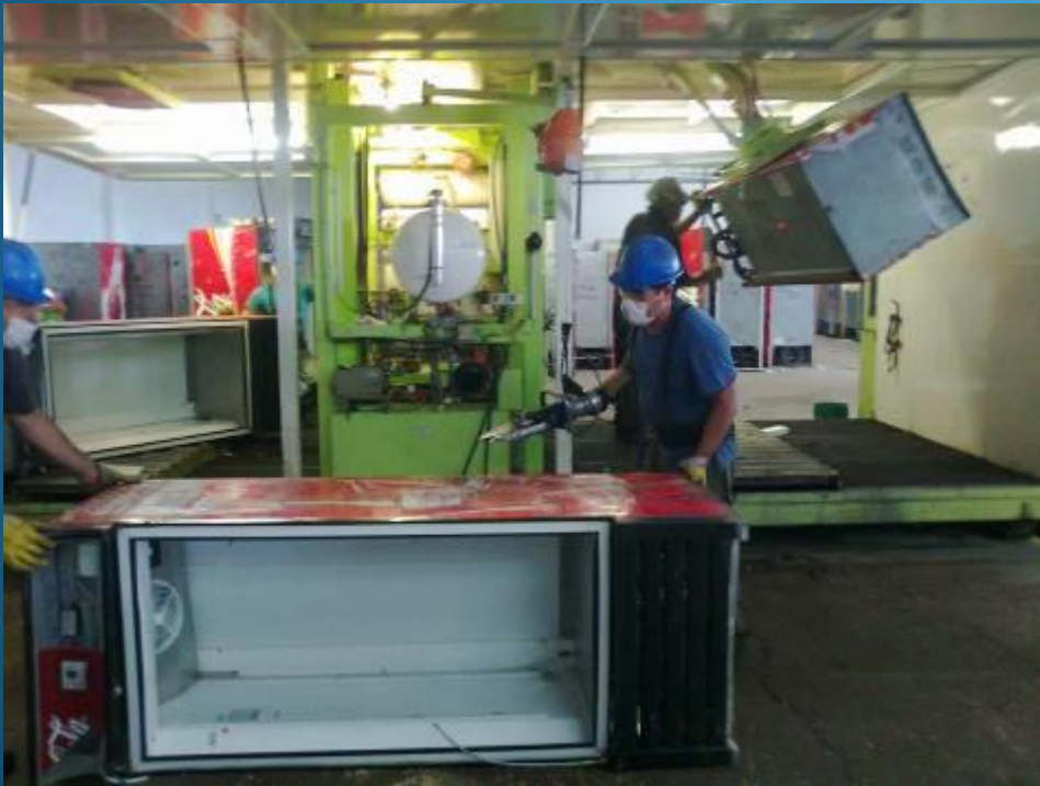
Refrigerants in a household dismantling facility
