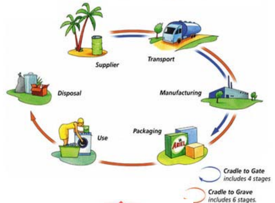
Fig 1: Structure of the Life Cycle Assessment ( LCA)
