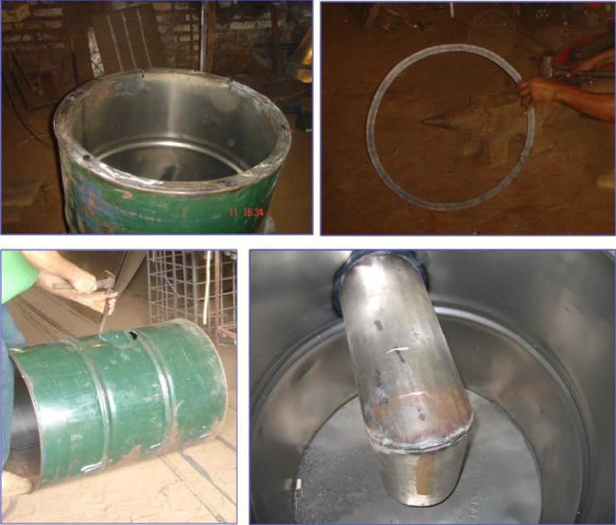
Fig. 4 Photographs of drum, upper mounting ring, and gas inlet
