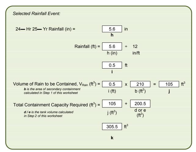
The volume of the secondary containment in  $\mathbf{c}$  is 315 ft<sup>3</sup>, which is greater than the required containment capacity in  $\mathbf{k}$  (305.5ft<sup>3</sup>). Therefore, the secondary containment is sufficient to contain the shell capacity of the tank and has sufficient additional capacity to contain a typical rainfall amount.
