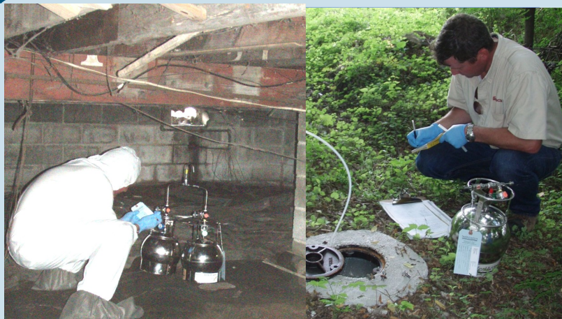
Vapor Intrusion Study: Crawlspace and Soil Gas Ports
