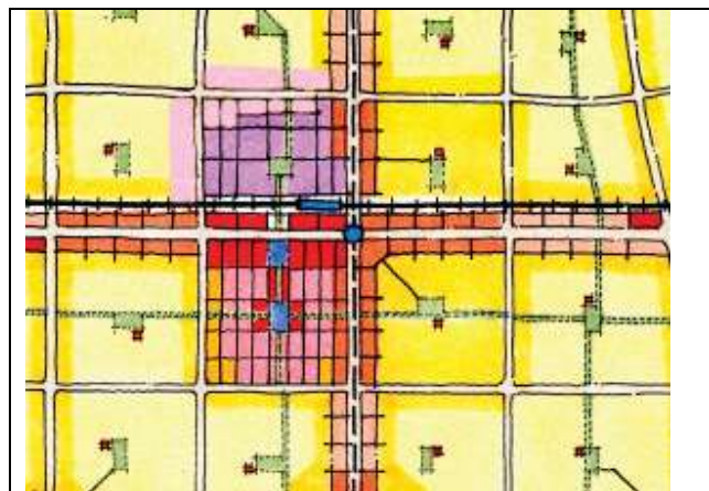
Figure 21. Conceptual diagram of a retail center (in red) located at one of the four quadrants of an arterial intersection. Image: Freedman Tung & Sasaki
