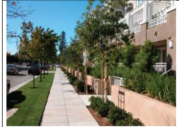
Figure 33. Sidewalk and view of private frontage in San Mateo, California. Layering of elements combine to create meaningful buffering for both pedestrians (curbside parking, planter strip, and street trees) and street-facing residences (decorative landscaping, additional trees, low wall, elevated grade change, stoop entrances, front setback, and front porch fencing).
