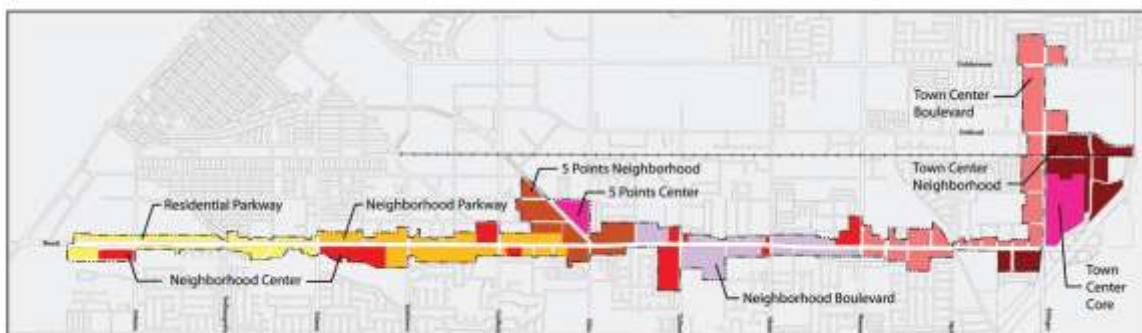
Figure 52. An example of a corridor regulating plan (Beach and Edinger Corridors Specific Plan, City of Huntington Beach, California). Image: Freedman Tung & Sasaki
