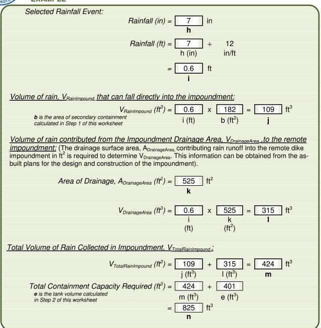
The volume of the impoundment containment in  $\mathbf{c}$  is 728 ft<sup>3</sup>, which is less than the required containment capacity in (825 ft<sup>3</sup>). Therefore, the impoundment containment is not sufficient to contain the shell capacity of the largest tank and the typical rainfall amount.
