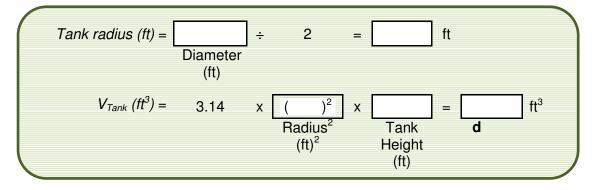
2b. Determine the volume of the largest tank when shell capacity is known,  $V_{Tank}$
