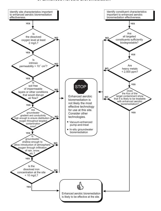
information in the corrective action plan, it should be possible to evaluate whether enhanced aerobic bioremediation is likely to be effective at the site.
