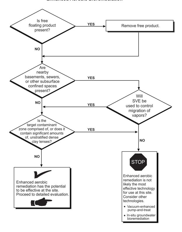
characteristics need to be evaluated. Next, the site-specific data must be compared to the criteria provided in the Exhibit to assess whether enhanced aerobic bioremediation is likely to be effective.
