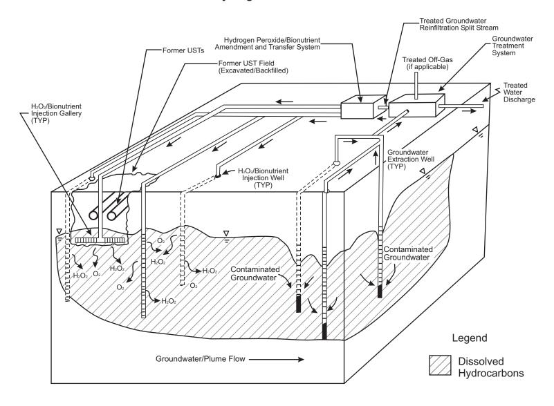
oxygen in groundwater (40-50 ppm). When this occurs, oxygen gas is formed, which can be lost in the form of bubbles that rise through the saturated zone to the water table and into the unsaturated zone.
