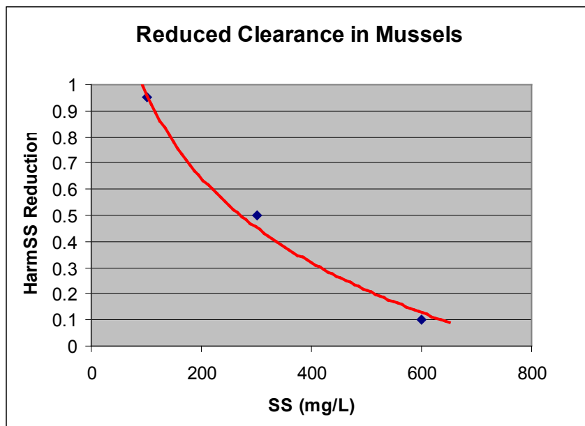
Figure 84. Reduction in clearance of sediment by freshwater mussels due to suspended sediments. Points represent supposed LC95, LC50, and LC10 values.
