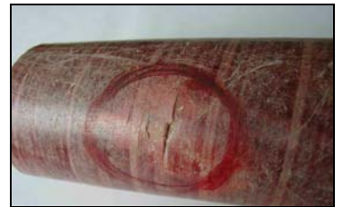
Fiberglass piping is cracked
