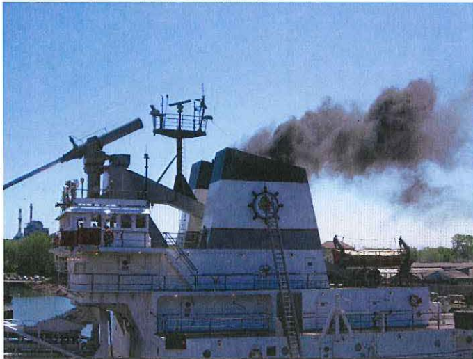
Figure 11: Another view of the vessel being loaded with 100% opacity smoke
