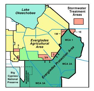
**FIGURE 35.** Location of Phase I phosphorus control program stormwater treatment wetlands. In combination with agricultural best management practices they are to decrease phosphorus to 50 ppb or less prior to discharge into the Everglades (adapted from SFWMD).
