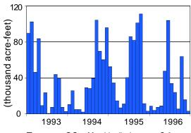
**FIGURE 22.** Monthly discharge at S-8. Discharge varies from zero to several thousand cubic feet per second in response to rain events.
