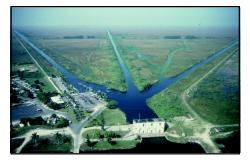
**FIGURE 11.** An extensive system of canals, levees, and water control structures has modified Everglades water conditions and provides a conduit for pollutant transport. This pump station discharges untreated stormwater from an urban basin into the Everglades.
