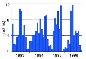
**FIGURE 20.** Monthly rainfall (inches) from 1993 to 1996 at S-8, a pumping station that provides flood control for part of the EAA by discharging into the Everglades.
