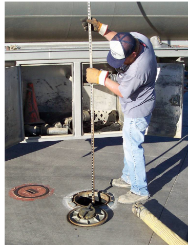
Measuring the product level in a tank
