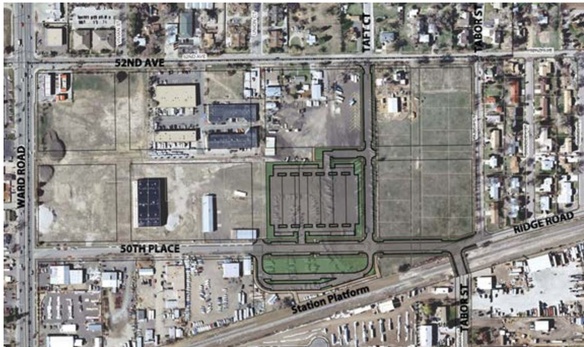
Exhibit D-8. Ward Road Station platform location and preliminary design. This figure shows the location for the station platform between 50 th Place and the rail line near Taft Court. The areas shaded in green indicate the station platform, the associated parking area, and street improvements to be funded with the station. Planned future street improvements are indicated as grid lines. Source: City of Wheat Ridge, Colorado.
