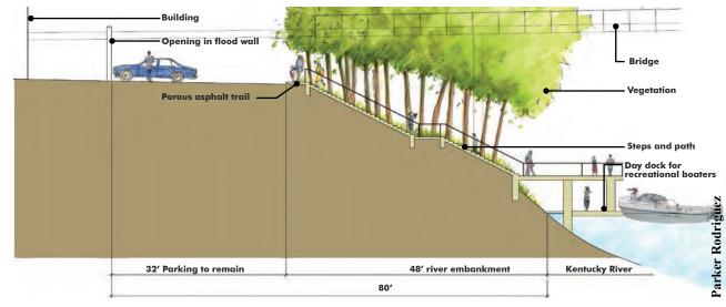
Figure 54: Design concept cross section for the western terminus of the river trail.
