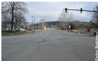
**Figure 23:** Main Street has large turning radii, creating an expanse of paving that is a challenge for pedestrians to cross safely. Cars travel at 30 miles per hour or faster through this intersection, making it hazardous for pedestrians and cyclists.
