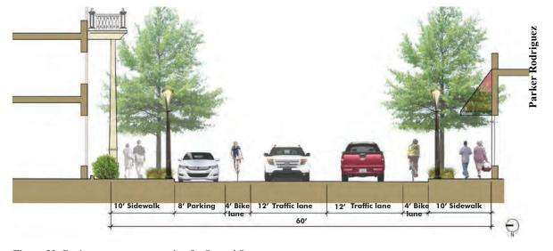
Figure 39: Design concept cross section for Second Street.
