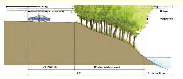
Figure 53: Existing cross section of the proposed trail along the Kentucky River at Bridge Street.
