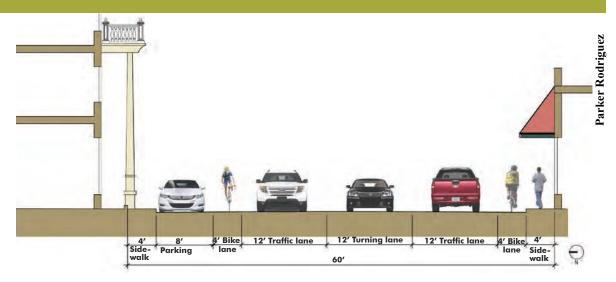
Figure 38: Existing cross section of Second Street between Steele and Shelby Streets.
