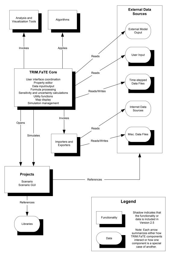
Figure D-1 TRIM.FaTE Computer System Architecture
