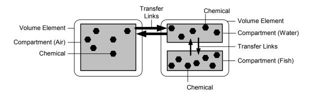
Figure 3-6 Transformation Links Between Chemicals within a Compartment
