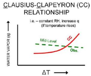
Figure 8. Clausius-Clapeyron (CC) relationship showing the required increase of water vapor as temperature increases at constant RH – red line. The observations of upper tropospheric water vapor – green dashed line – do not follow this theoretical relationship.
