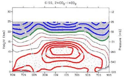
Figure 10. North-South vertical-cross section showing Hansen's early GCM's model change in temperature (oC) that would accompany a doubling of atmospheric CO2. There is no way a doubling of CO2 and an extra 3.7 W/m2 blockage of OLR to space could lead to such extreme upper tropospheric temperature rises. These large temperature increases occurred because of Hansen's unrealistic upper level water vapor assumptions.
