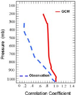
Figure 4. Comparison of correlation coefficient between upper and lower level tropospheric water vapor of the typical GCMs output (red) and that of the Rawinsonde-reanalysis observations (blue line). The GCM outputs are programmed to have a
