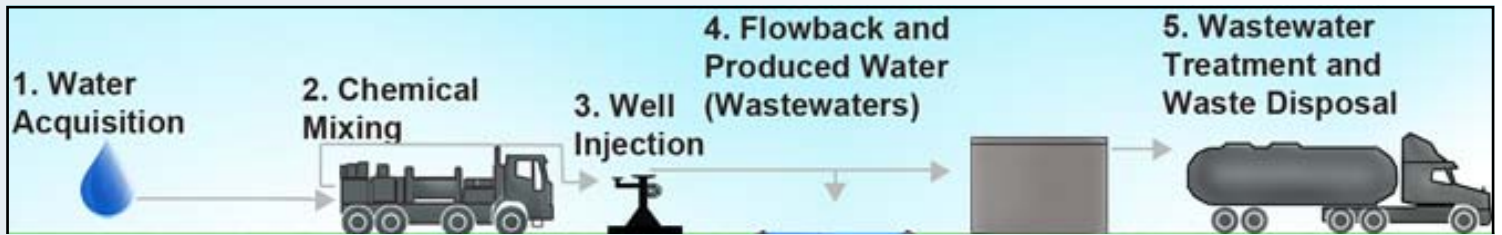
The five stages of the water cycle as pertains to the hydraulic fracturing process.
