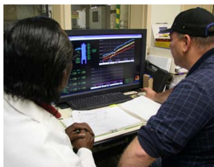
EPA engineers at the 1.2 megawatt Multipollutant Control Research Facility in North Carolina can burn coal, oil and gas under different operating conditions to test a variety of different pollutant control technologies.
