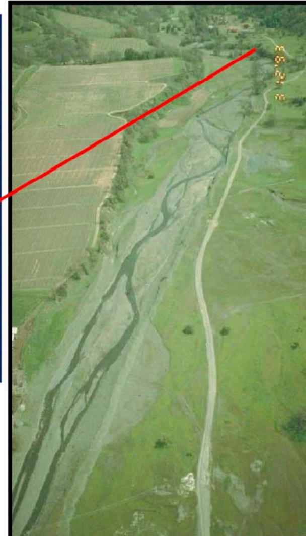
Figure 5: Alluvial fans are areas of high infiltration of surface flows into groundwater and are not good locations for gaging stations
