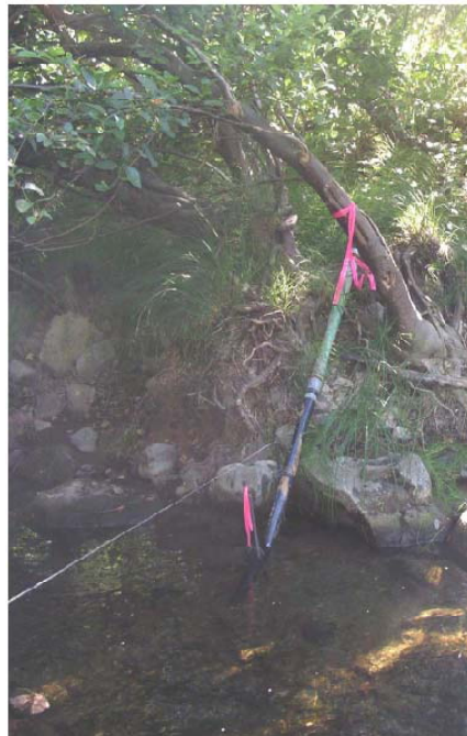
Figure 14: Pressure transducer in plastic pipe housing
