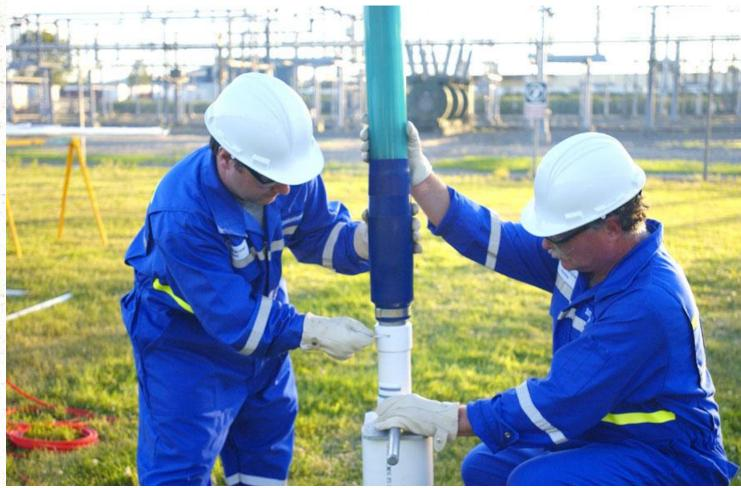
Schlumberger Westbay System is one commercial sampler option Uses packers to isolate zones, with independent pumping and sampling ports Can be removed and reused elsewhere
